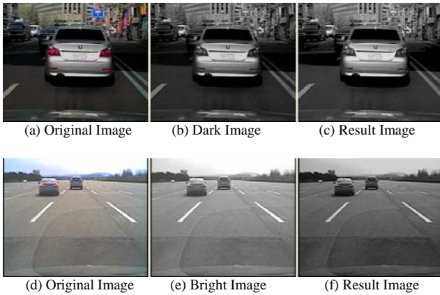
Fig. 2 Auto intensity control considering the image brightness
